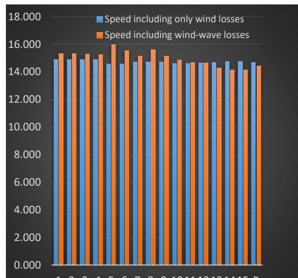
Figure 9. Comparison diagrams of wind-wave losses without regard to flows and with them:
