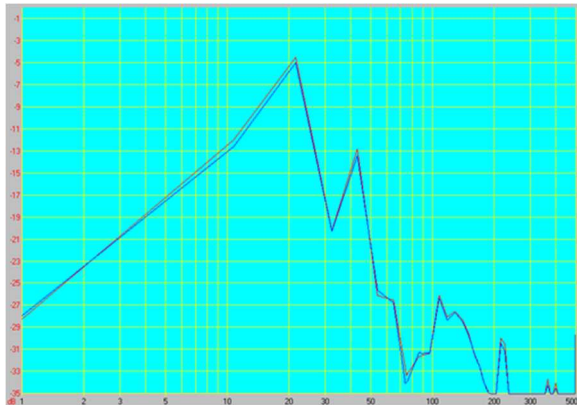
Figure 2. Amplitude-frequency response characteristic of a vibroacoustic signal recorded during the tests of a milling machine model with a new antifriction bearing
