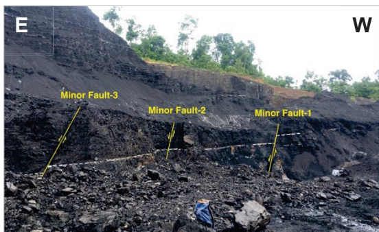
Fig. 5. Minor faults in the mine pit (blue bag as parameter).
