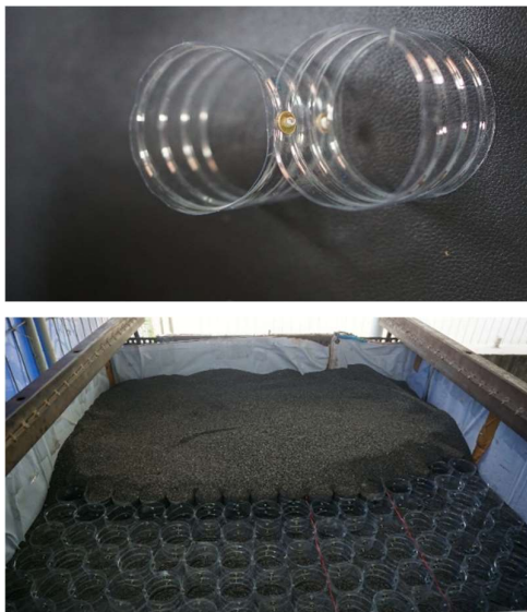
Fig. 1. Geocell plastic bottle waste
