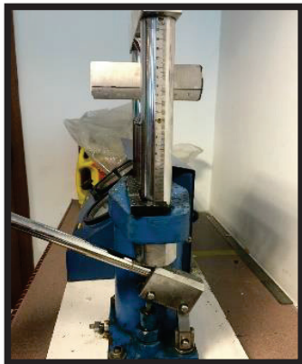
Fig. 7. The point load index test from the side view.
