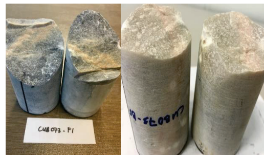
Fig. 9. Samples from CUB 073 and fractured after point load test.
