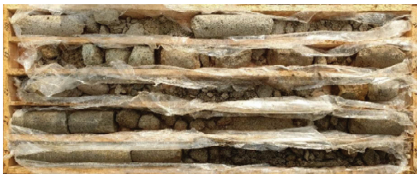
Fig. 7. Typical drill cores at the research location, material lapilli tuff with medium quality
