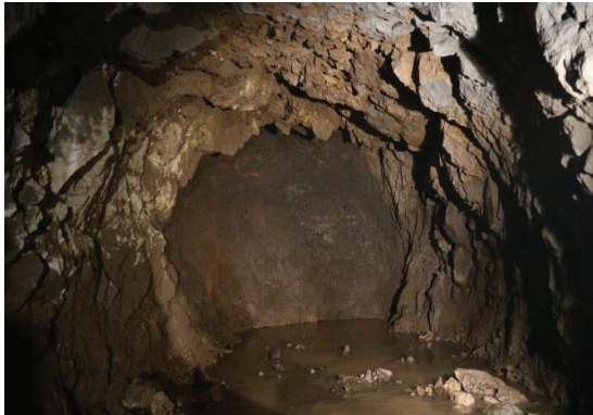
Fig. 6. Fresh to slightly weathered andesite.
