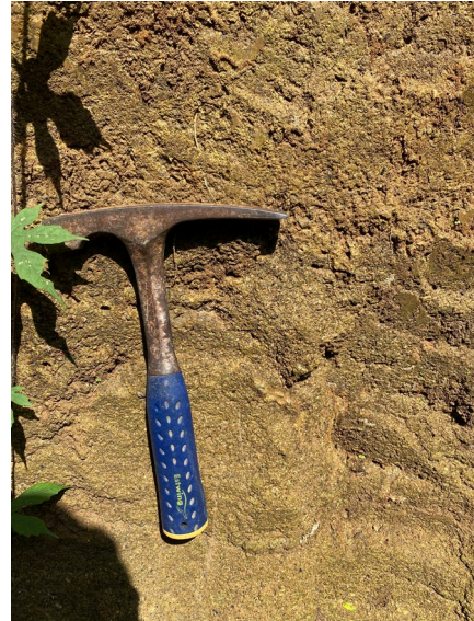
Fig. 5. Moderately weathered tuff lapilli.
