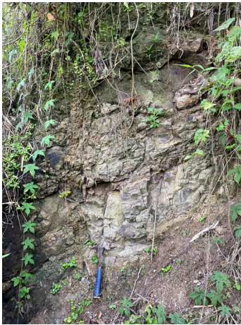
Fig. 3. Slightly weathered tuffaceous sandstone.
