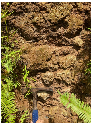
Fig. 4. Moderately weathered andesite breccia.
