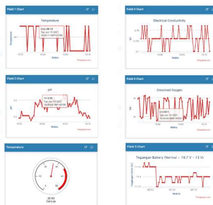
Figure 7. Display of water quality and battery voltage monitoring on a smartphone/PC.
