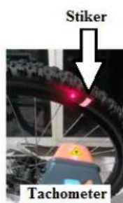
Fig. 5. RPM measurement using tachometer.
