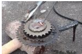
Fig. 3. Free wheel welding to front chainwheel
