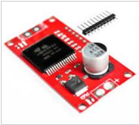
Fig. 5. Motor Driver VHN2SP30 (Source: cdn.instructables.com )
