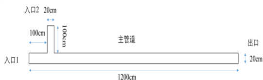
Fig.1 Schematic diagram of the pipeline model
