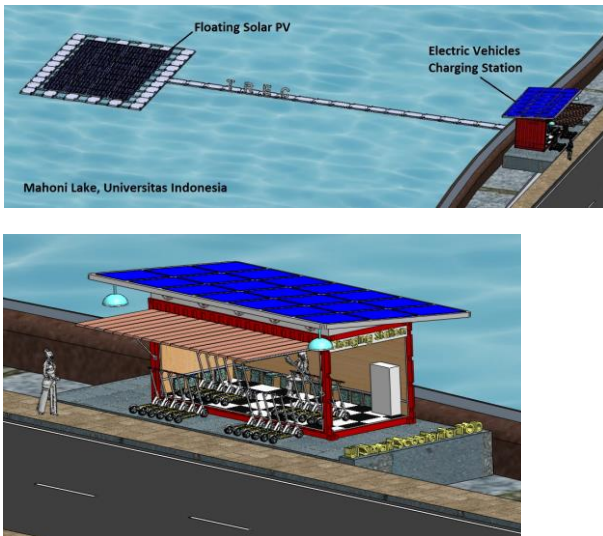
Fig. 6. Electric Vehicles Floating PV Charging Station
