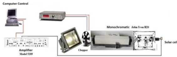
Figure 1. Measuring bench (IPCE) for measurements of the external quantum efficiency (QE).
