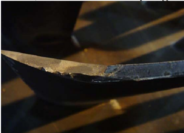
Fig1. Sectional appearance of compressor blade
