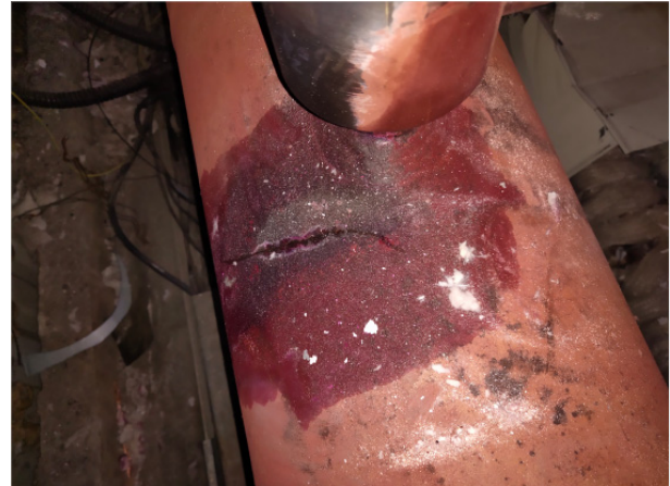
Fig6. Circumferential cracking of the base material of heating and desuperheating pressure reducer pipe.
