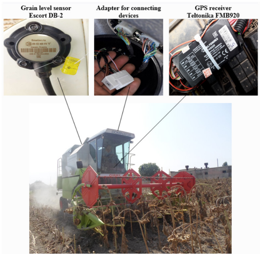
Fig. 2. Outlook of the adapted combine harvester equipped with GPS receiver, grain sensor.
