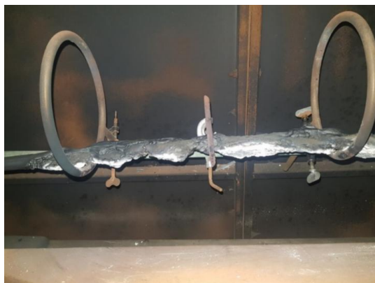
Fig. 3. Appearance of VVG non-combustible(A) - FRLS 3*10 cable sample after test.
