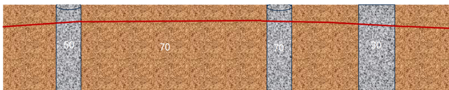
Fig.8 vertical deviation of borehole
