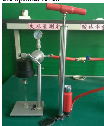
Fig.3 test of slurry water loss
