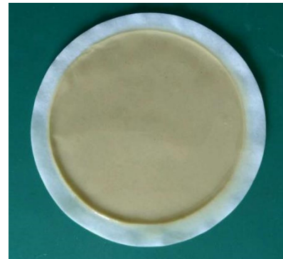
Fig.4 dense mud cake obtained after slurry water loss
