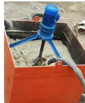
Fig.5 preparation of test slurry
