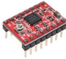
Fig. 9. Exterior view of the Pololu A4988 stepper motor controller.
