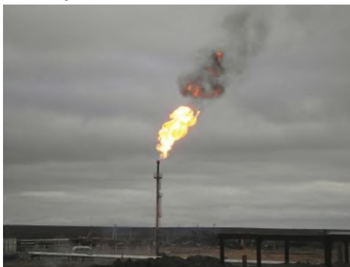
Fig. 2. Working gas torch.
