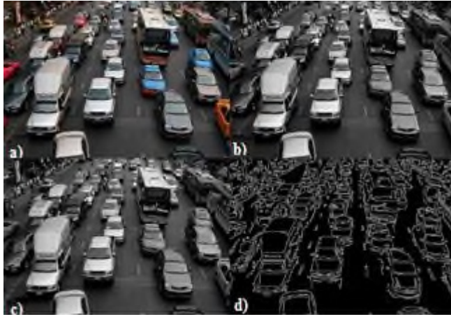
Fig. 1. Converting the resulting video from a surveillance camera: a) Splitting into frames. b) Image discoloration. c) Image enhancement. d) Detection of vehicle edges.
