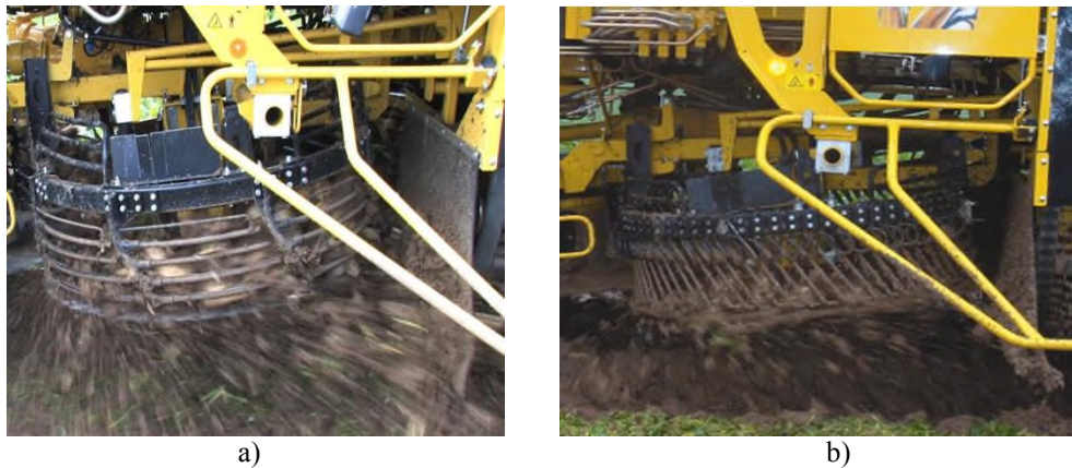
Fig. 2. The working process of cleaning root crops: a - with favorable; b - unfavorable conditions (using sieve springs)
