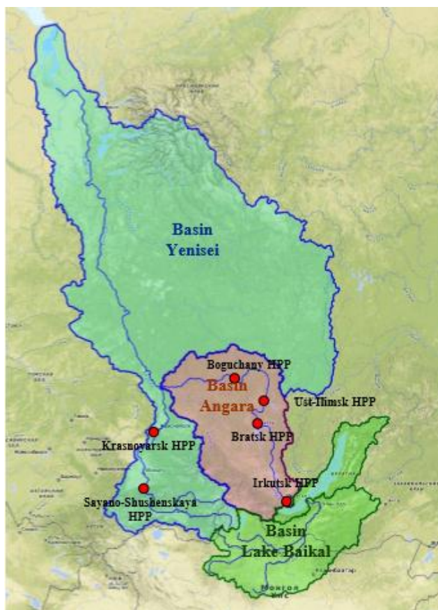
Fig. 1. The scheme of the Angara-Yenisei HPP cascade
