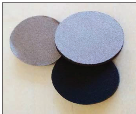
Fig. 2. Textile electrodes without edging.
