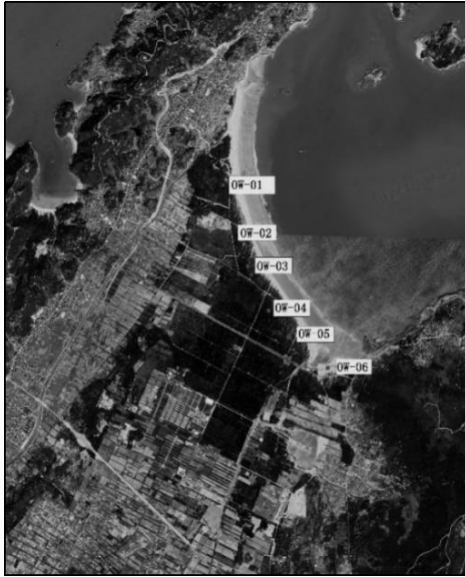
Fig.4. Simulation range and observation well layout of Luyangpu underground reservoir
