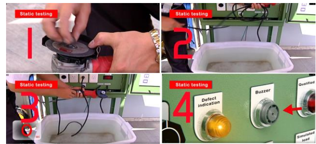
Fig. 4. Static power consumption inspection process for portable electrical equipment.
