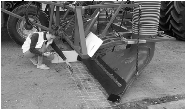
Fig. 2. Taking of air flow speed readings in front of the nozzle.
