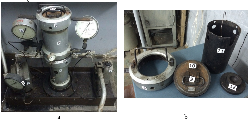
Fig. 1. Volumetric compression chamber Azimuth 85D01B: a - the lower part; b - the upper part.
