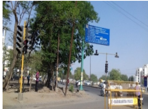
Fig. 4 Sign board post at turning obstructs vehicles
