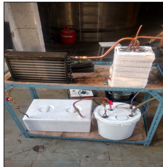
Fig. 5.8. Experimental setup of VARS using solar thermal energy
