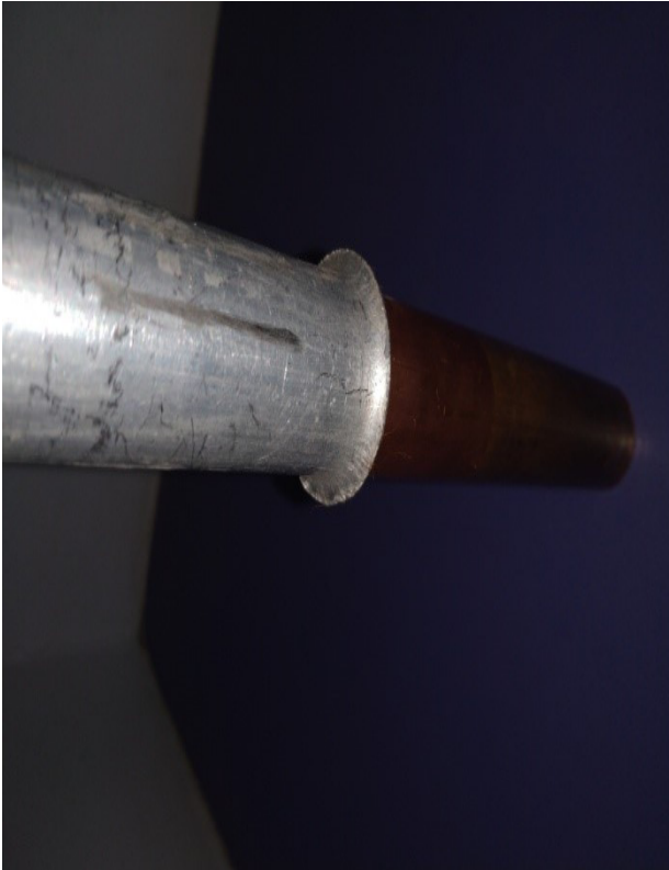
Fig.1.0 First two trailsrunAA6063- Cu Failed
