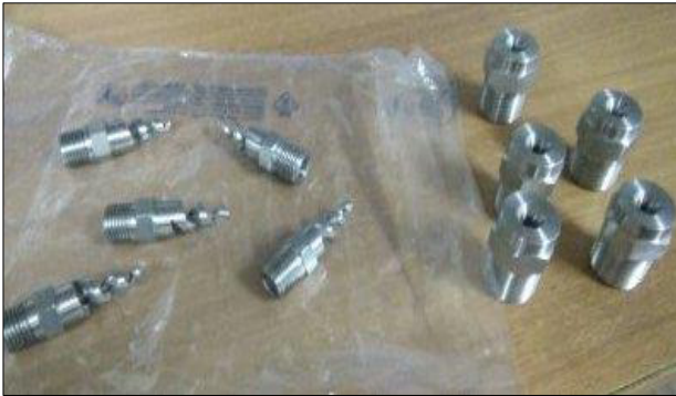
Fig. 7. Full cone and spiral nozzle (spray angle: - 90°)
