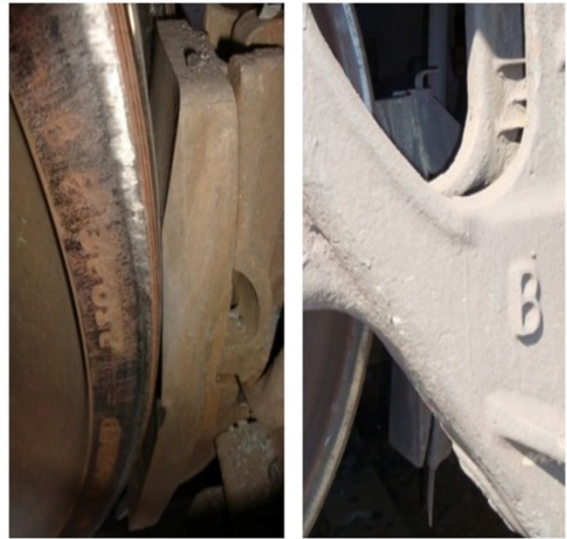
Fig. 1. View of a dual wedge-worn brake pad in operation.
