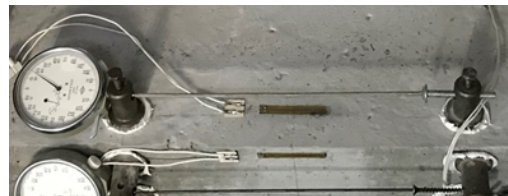
Fig. 9. The location of the strain gauges under the indicator.
