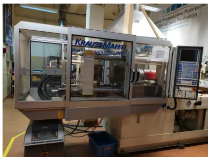
Fig. 1. KRAUSS MAFFEI KM65 - 160C1 injection molding machine
