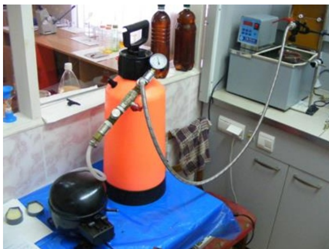
Fig. 4. Experimental installation for determining the influence of spray parameters on the alkalinity of methyl ether.
