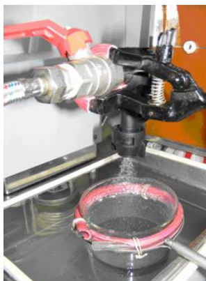
Fig. 6. Spraying aqueous solution of 1% citric acid in the test sample of methyl ether.
