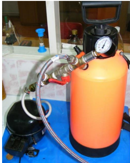
Fig. 5. Hydraulic pump on the basis of garden sprayer and refrigerator compressor.
