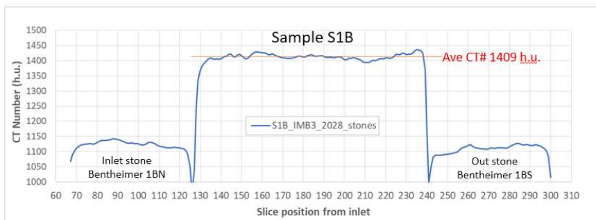
Fig. A2. Profile of average X-ray CT numbers through the assembly of inlet stone-sample-outlet stone mounted in the test rig, prior to commencing measurements. The sample has a uniform brine saturation of 30% and is in capillary equilibrium with the stones. The dip in CT number at the boundary marks the position of the single ply Kimwipe tissue used to maintain good continuity of the brine phase between the end faces of rocks.
