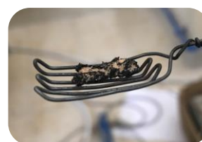
Fig 5. The residue after combusting straw pellet at 850 °C, tests were carried out in a stream of inert material at G_s = 2,5 \text{ kg/m}^2\text{s} .
