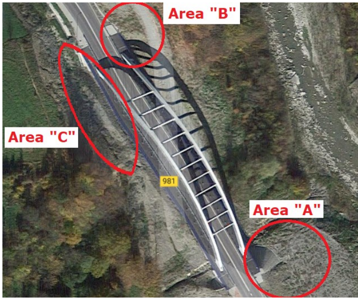
Fig. 4. Areas of research adopted for differential analysis with a terrestrial laser scanner.
