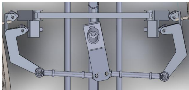
Fig. 5. Steering system using regular tie-rods.
