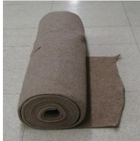
Fig. 7. Polypropylene and coir fibers as non-woven fabric.
