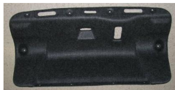
Fig. 9. Trunk lid made using non-woven fabric composite felt
