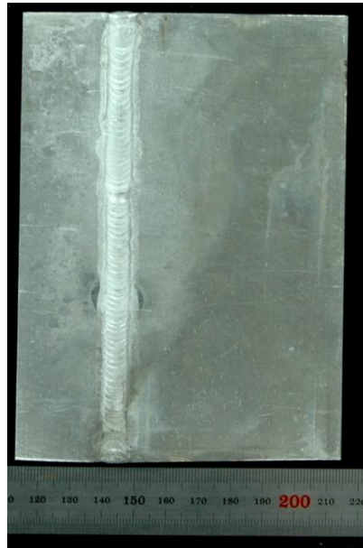
Fig. 1. The welded plate by TIG on the longitudinal direction.
