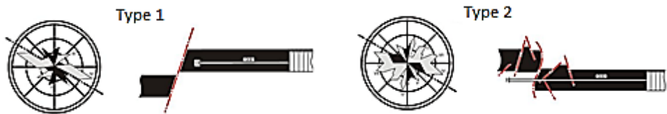
Fig. 2. Typical forms of tectonic disturbances of types I and II and associated systems of cracks
