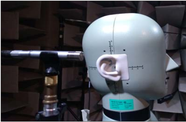
Fig. 4. The microphone n° 3 near the ear of maniquine in the chamber room
