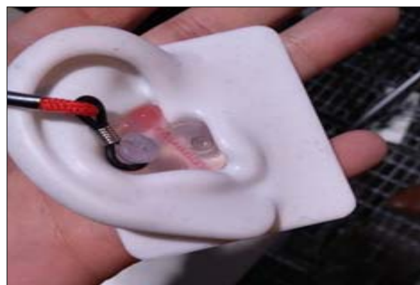
Fig. 2. HPD type C inside the ear of mannequin
