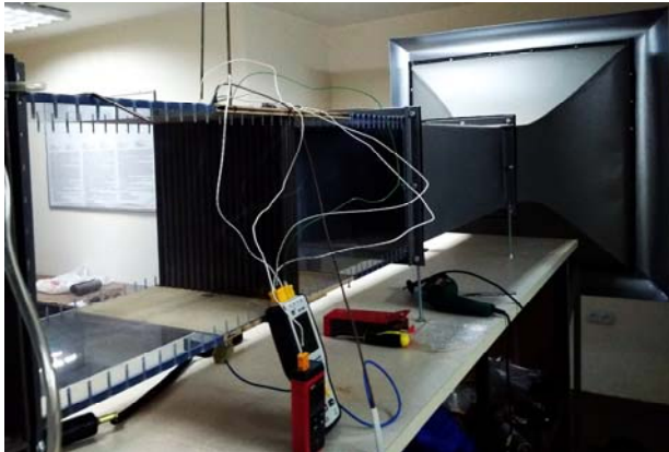
Fig. 1. General view of open circuit section type wind tunnel of subsonic speeds
