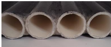
Fig. 1. Ceramic piping of the solar collector developed at the Białystok University of Technology in the Department of HVAC Engineering.
