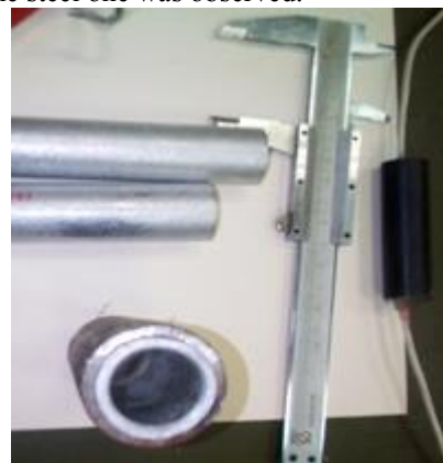
Fig. 5 - Flared aluminum tube in steel pipe
