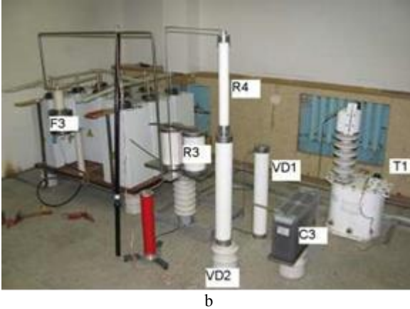
Fig.1. a) Installation diagram: Tr - high-voltage charging transformer, B - high-voltage rectifier, C - shock capacitance, K - switch (spark discharge), T - technological node; 1 - electric blasting cartridge, 2 - steel tube, 3 - copper tip, 4 - aluminum tube b) Photo of the installation
