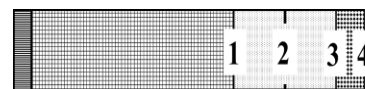
Fig. 2. Schematic diagram of a wall section, whereby 1 is located between the concrete block and insulation layers, 2 is the middle of insulation layer, 3 located between the insulation and gypsum board layers, and 4 is the inner surface.
