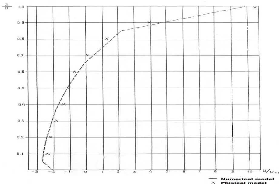
Fig. 3. Comparison of experimental data and numerical modeling for the wind current in the channel.
